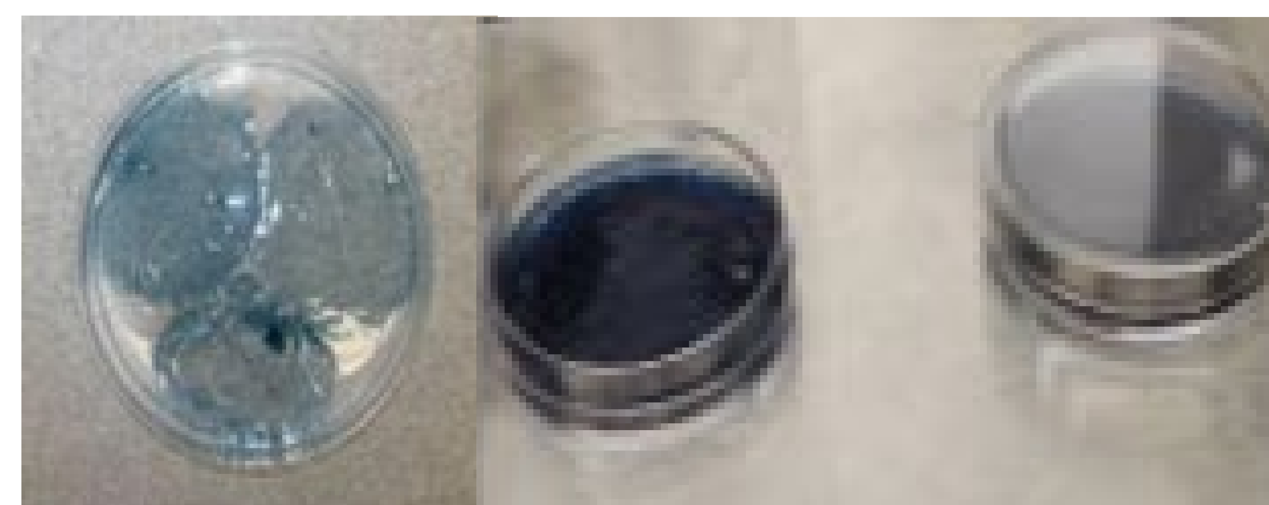
Figure 6. Left hand side of image shows initial hydrogel fabrication that contains a light blue color. Right hand side of image shows final hydrogel fabrication which contains a dark rich blue color.
