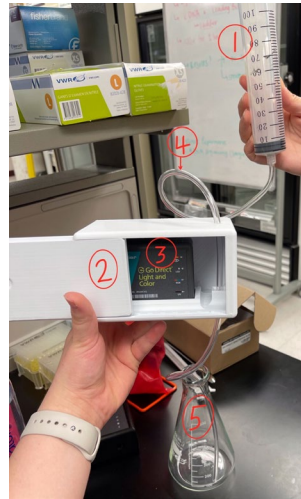
Figure 3. Model of device with light sensor and syringe
