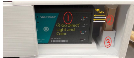
Figure 4. Model of device with light sensor and cuvette placement
